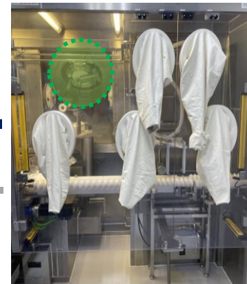
RTP port from the outside
