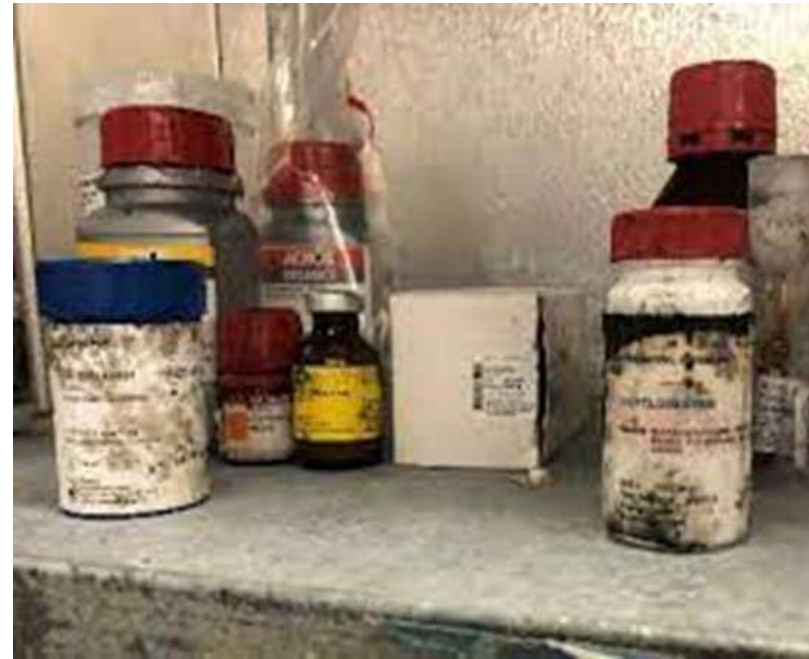
Mold on labels in coldroom
